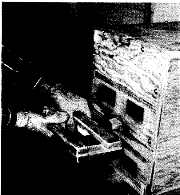
Fig. 16. The Pump Handle of the Durability-Test Pump, showing how one man best holds it when two men are pumping.
